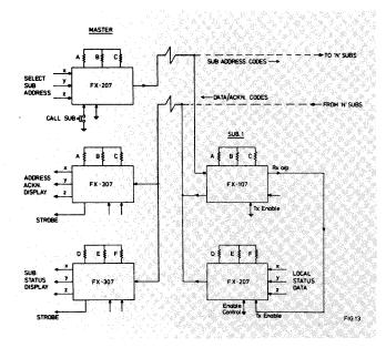
Sophisticated signalling functions are easily implemented using '07 series devices. Fig. 13 outlines a system where remote sub-stations are selectively addressed, receipt of an address verified and the sub-station status displayed.
