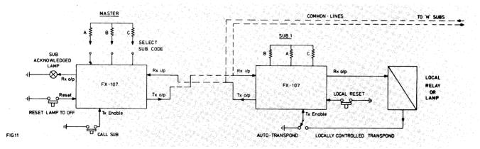
Fig. 11 shows a simple master/sub-station calling system employing FX-107's. Sub-station address codes are selected by switching RA/B/C at the master; receipt of an address code operates a local sub-station switch function.
