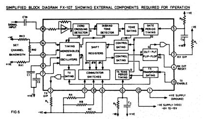
The FX-107 functions as either a receiver (RX) or a transmitter (TX); simultaneous operation in both modes is not possible. The rules are:
