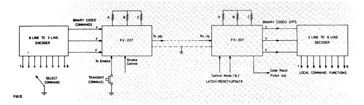
Fig. 12 shows how a FX-207 and a FX-307 can be used to transmit several coded instructions to a remote point, using one common line.
